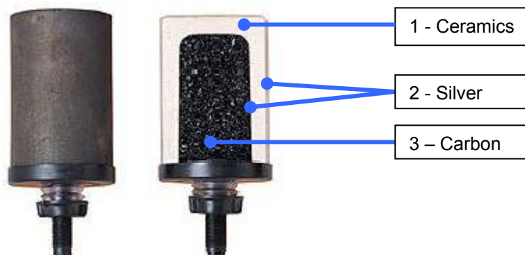
Figure 1 : 3 layers of Stefani filter candles
